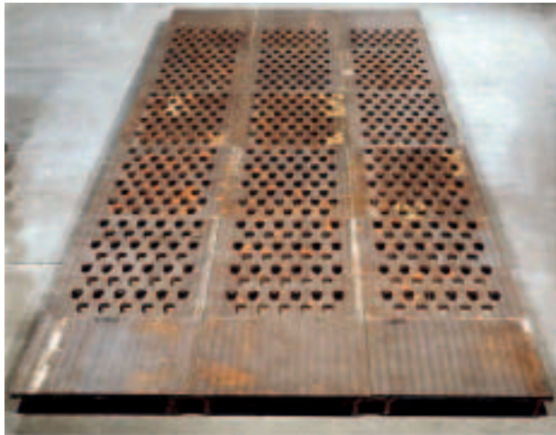
Bild 8: Siebbelag aus V-100-Verbundplatten Fig. 8: Screen liner made of V 100 compound wear plates
